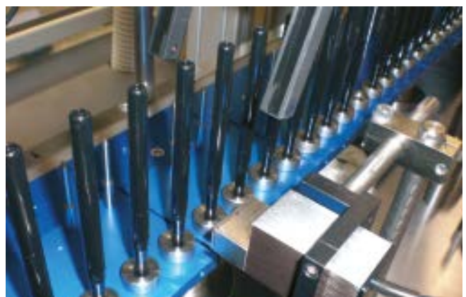
Precise application of oil on plastic parts
