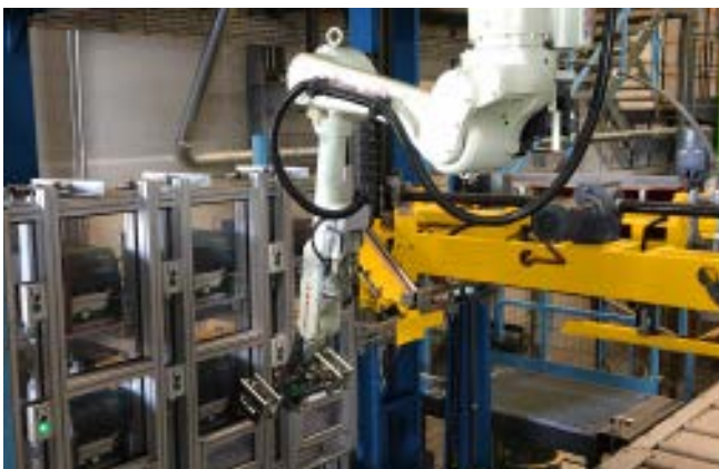
Flexible robot labeling system
