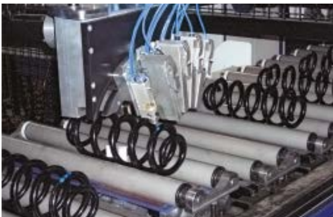
Marking of steel springs for type classification
