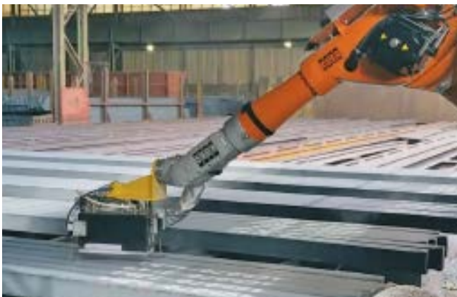
Marking of steel billets - spray mark block on robot
