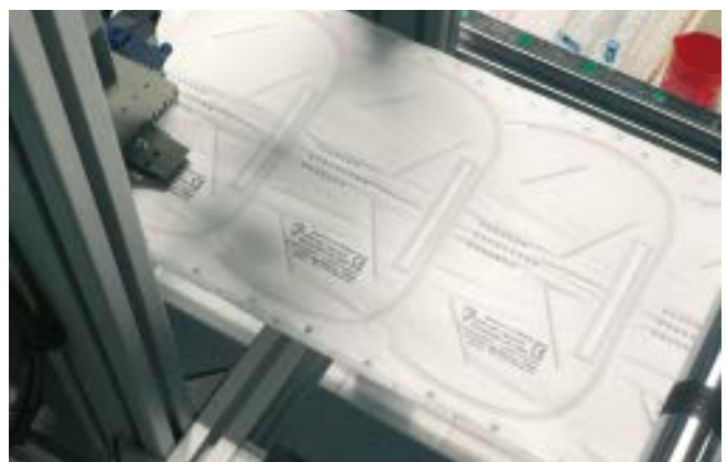
Multi-line marking of FFP2 respirator mask
