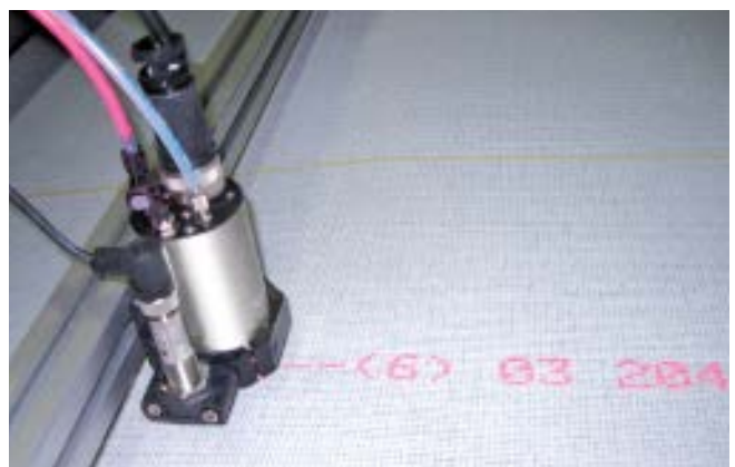
Coding and marking of sheeting materials
