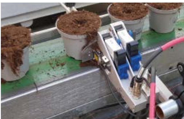
Direct marking with the EU plant passport
