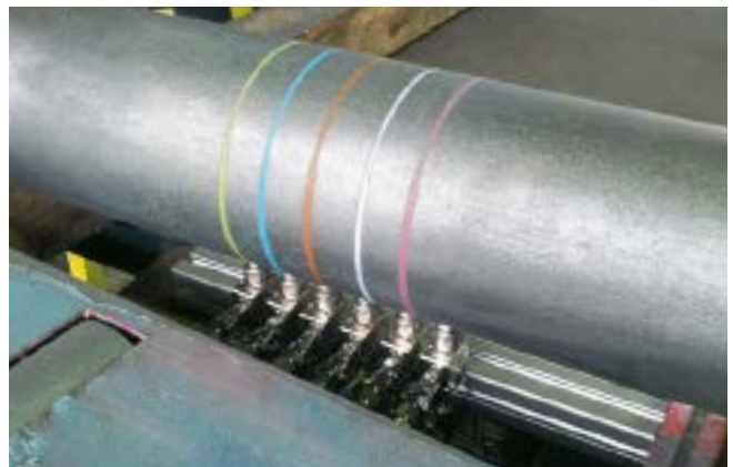
Ring marking of steel pipes
