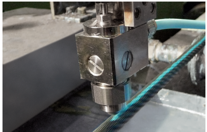
Color marking of wire cables
