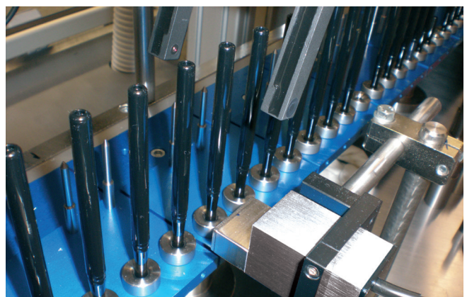
Precise application of oil on plastic parts
