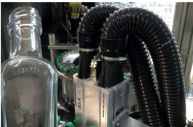
Coding and marking of glass with CO 2 laser IP65
