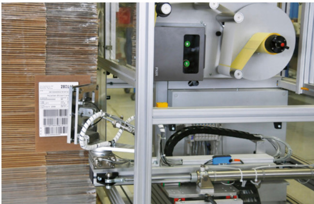
Applying labels to stacks of corrugated cardboard
