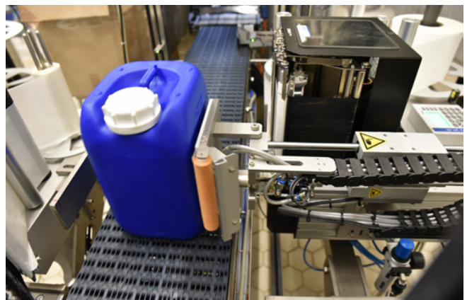
Labeling of canisters
