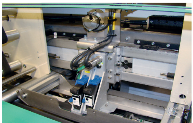
HR pro OEM integrated in inserter machine
