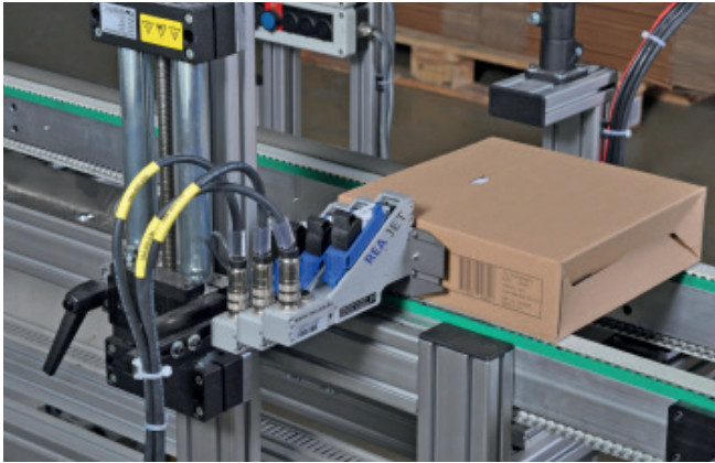
HR pro OEM integrated in packaging line
