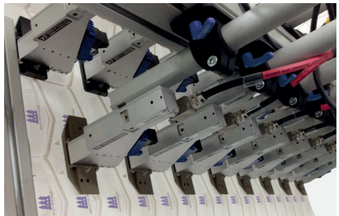
Label finishing with 16 HR print heads
