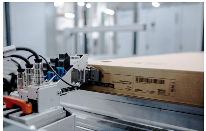
Label replacement with 3 REA JET HR print heads
