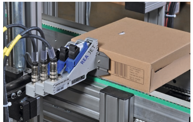
Marking cardboard boxes with barcodes
