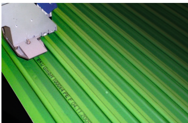
Coding of plastic profile plates
