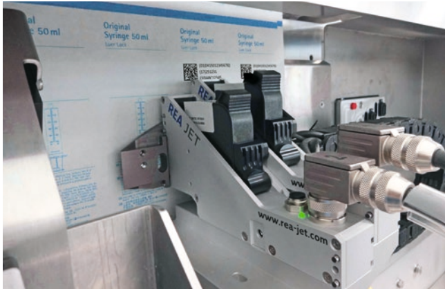
UDI marking of packaging material
