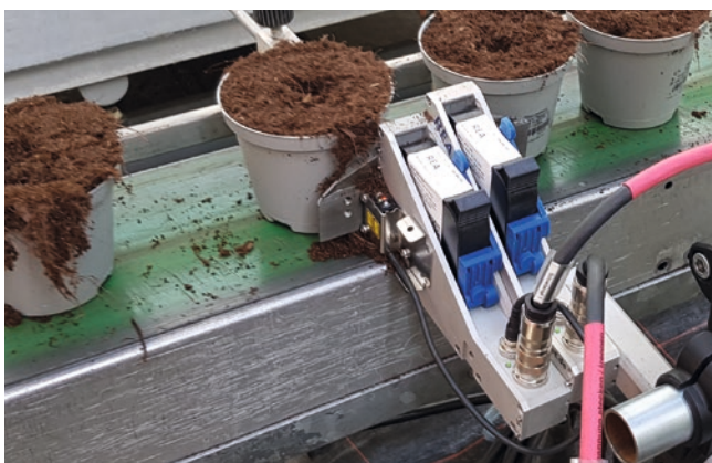
Direct marking with the EU plant passport
