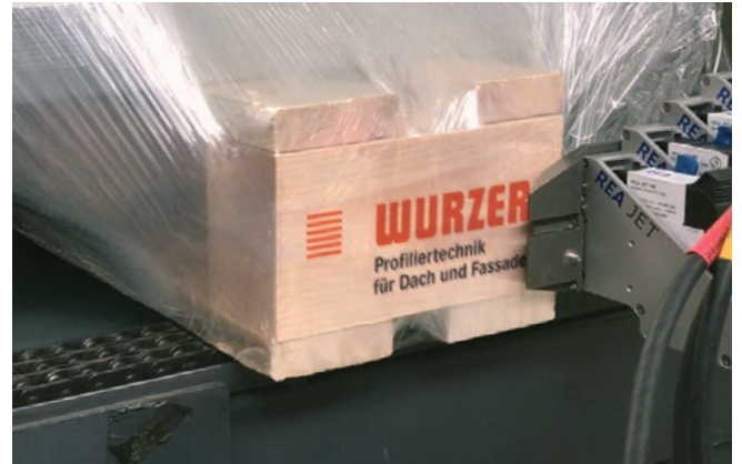
Two-colored marking of foil
