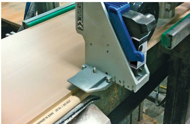
Coding and marking of laminate
