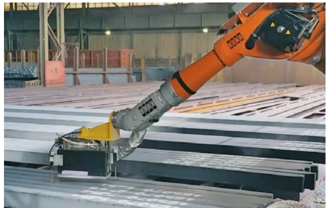
Robot controlled billet marking with high temperature paint
