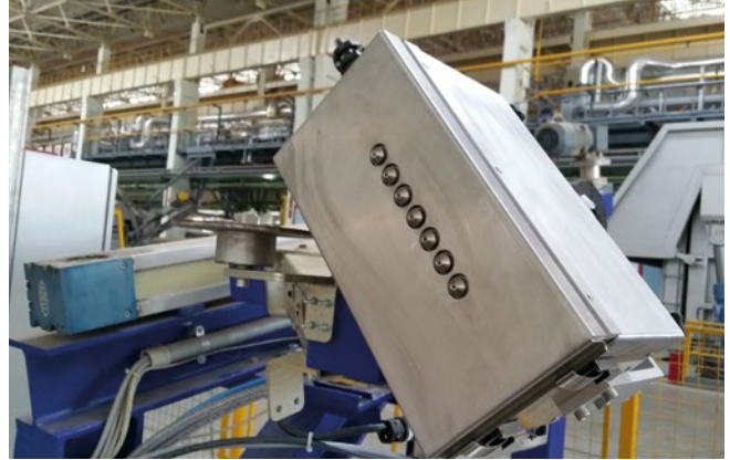
Protective housing SRP-10 for rough environment
