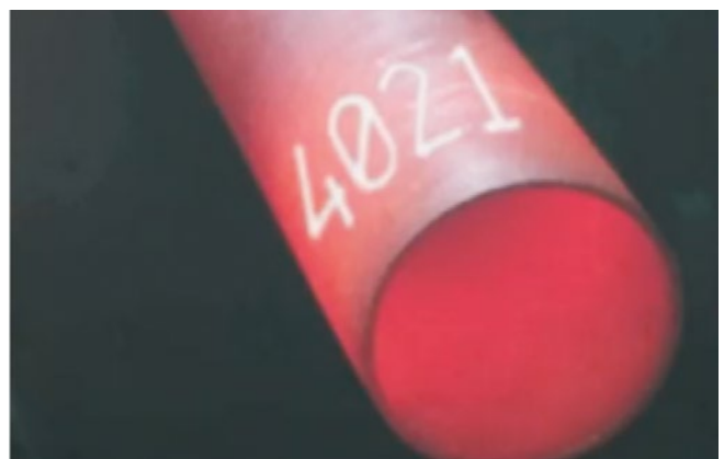
Marking of red-hot steel with high temperature paint
