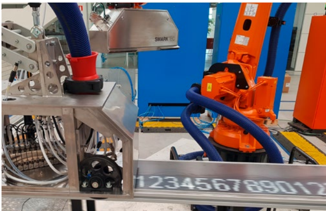
SRP-10 spray mark block for marking sheet metal
