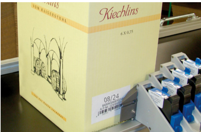
Label replacement on wine cartons (REA JET HR)
